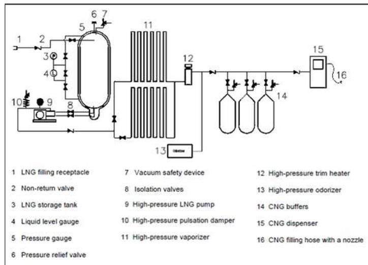
Figure 2-9 LCNG Station. Source: GNVERT
