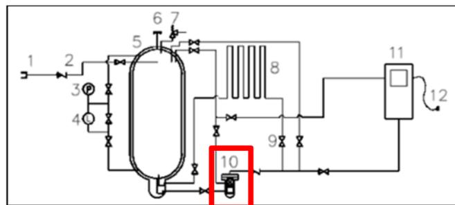
Figure 2-2 LNG Station scheme and location of the cryo-pump. Source: GNVERT
