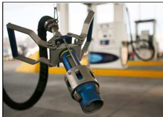
Figure 2-5 LNG fuelling nozzle. Source: NGVA
