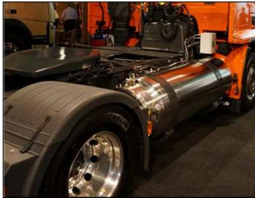
Figure 2-8 LNG truck: Iveco Stralis. Source: Iveco
