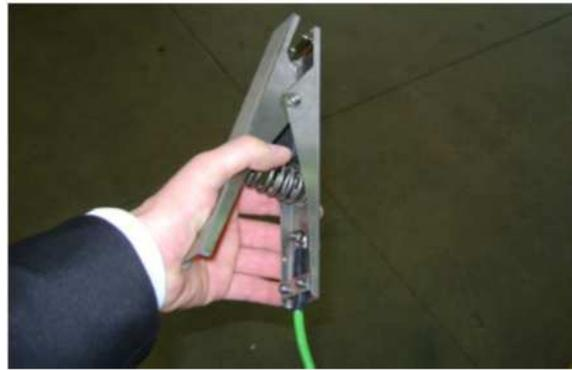
Figure 4-2 Earth cable / clip. Source: BOC
