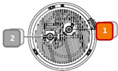
3. Check the pressure on the manometer. This should indicate upper 8.5 bar.
