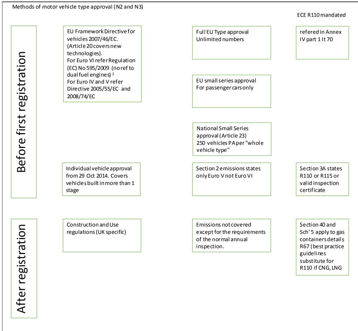
Figure 4-8 Methods of motor vehicle type approval (N2 and N3) from Hardstaff
